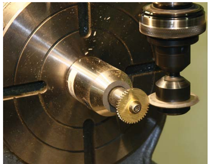
13. Cutting a gear.
