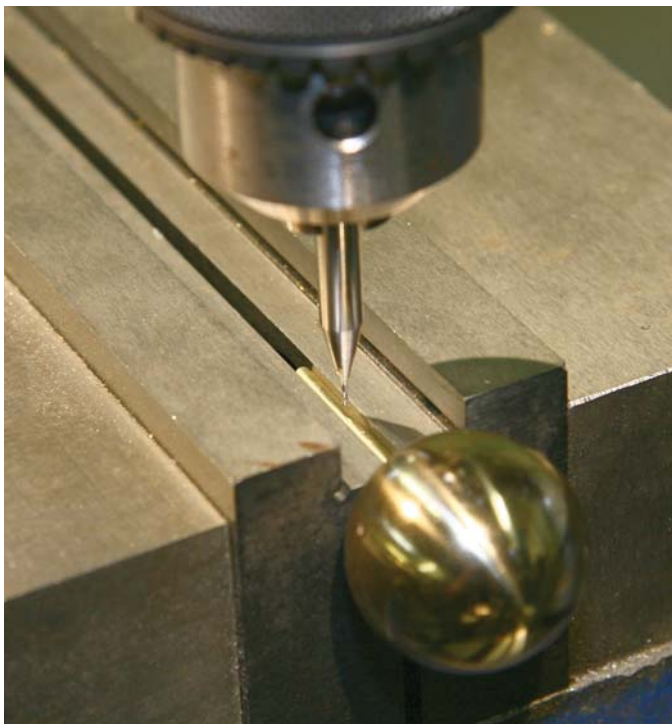
22. Drilling the Sun shaft.
