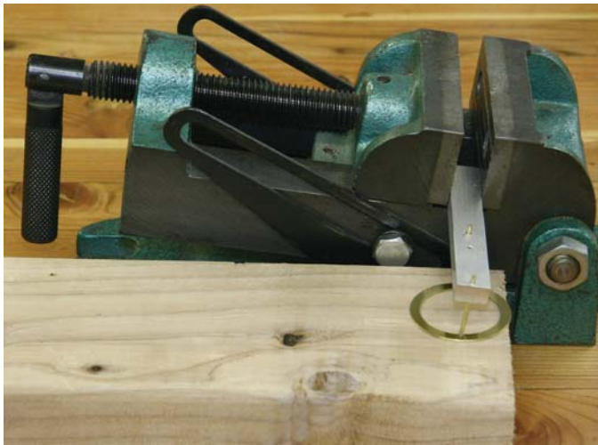
21. Soldering the ring supports.
