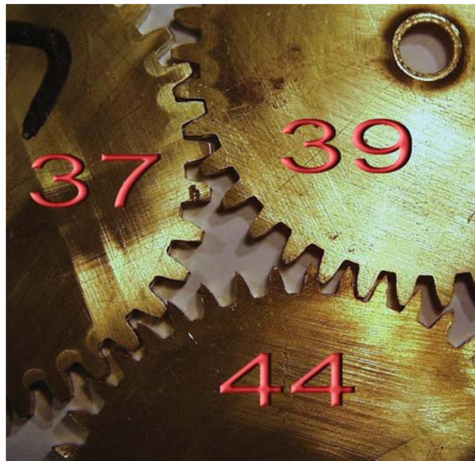
**Figure 27. Meshing of the gears.**
